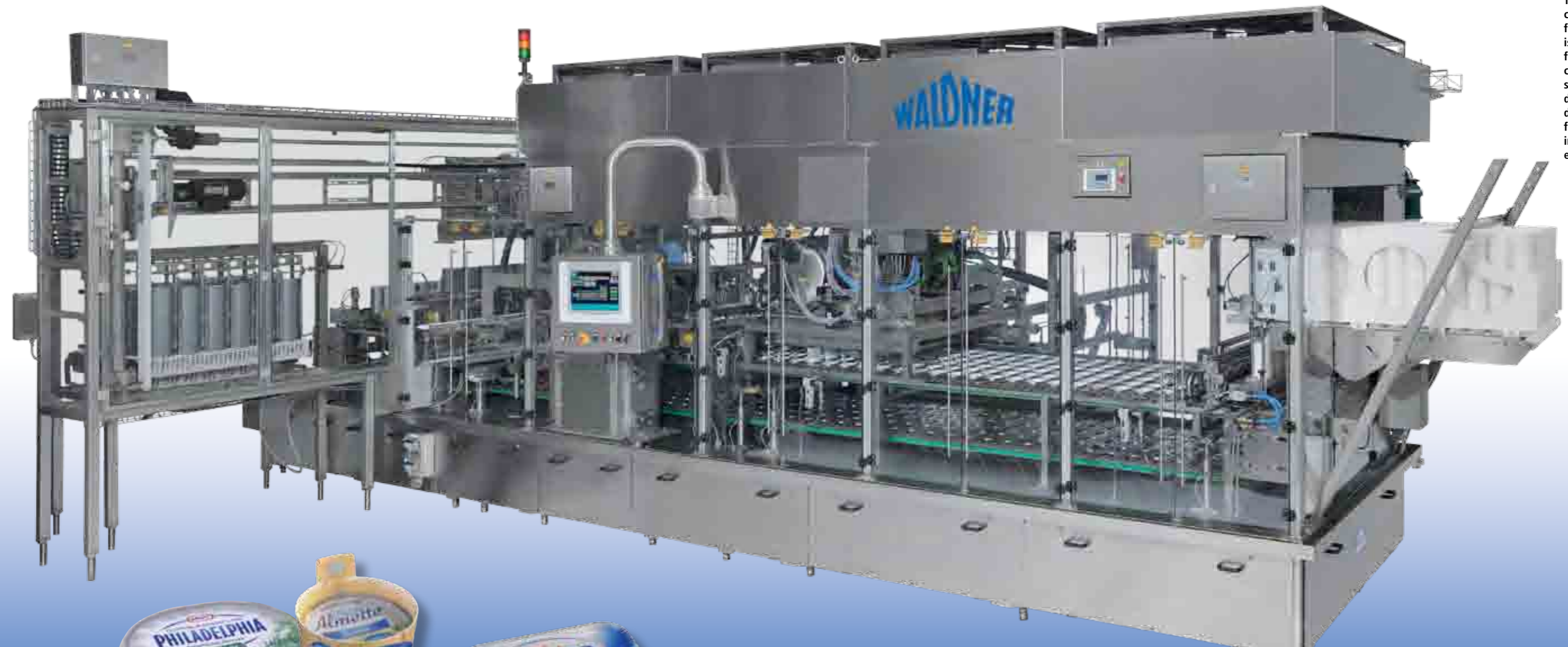
The WALDNER cassette system for cup stockpiling is an extremely flexible way of creating a high storage capacity despite having to deal with various formats, sometimes incompatible with each other.
