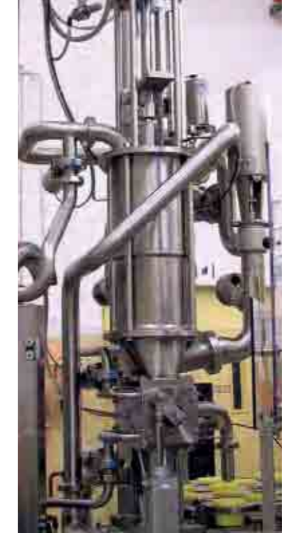
Compensation cylinder for synchronizing product feed and discontinuous filling process
