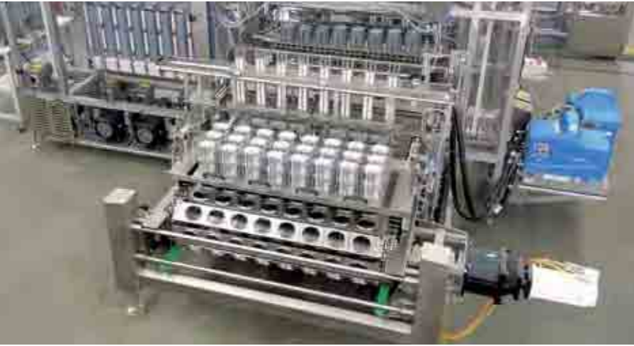
The stacking of filled and sealed cups is done in stacks of five for collection by the robot gripper at the final packaging.
