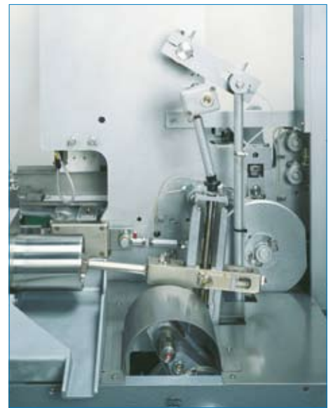
Drive of dosing station
