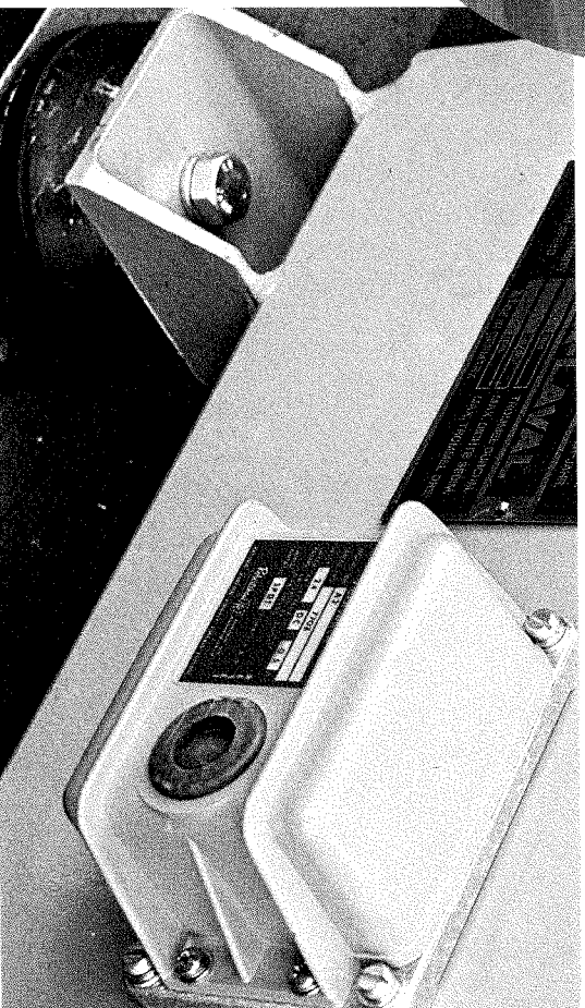
Power cutoff switch operated by opening of the vessel.
