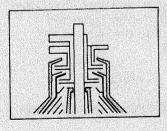
Many separators are equipped with paring disc liquid discharge. It is important that the paring device/feed tube assembly has correct height adjustment and is securely tightened before machine is operated. See instruction manual for detailed instructions.
