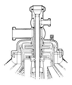
The separator is equipped with paring discs:
