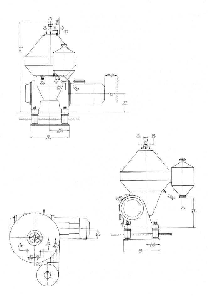
The separators are used for separation, standardization and purification of hot milk. They are constructed for continuous, automatic operation and CIP cleaning.
