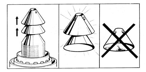
Inspect **all** discs. The upperside as well as the underside of **every** disc must be bright. Fatty discs and sediment residues on the discs indicate bad cleaning.
