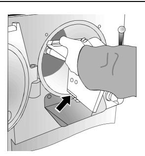
When reassembling the beater, catch it with both hands and push the sliding shoes in order to insert it easily. Push to the beater to the bottom and at the same time let it turn in order to fully insert the beater shaft into its seat.
