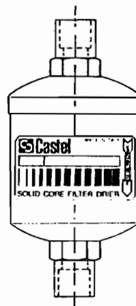
Attacchi a saldare ODF - OOM ODF - OOM solder connections
