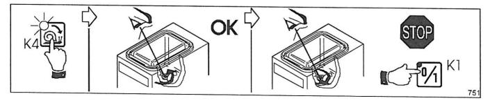
press the SLOW BEATING ACTION button [K4] and observe BEATER rotation. If it is ANTICLOCKWISE (as shown in the drawing) the machine is connected correctly and is ready for use;
