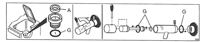
Occasionally check the choke ring [A] and the washers [G] shown in the drawing. Replace them if broken, worn or dilated (in the latter case washers tend to come out of their sockets).
