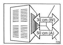
Place the device on the floor, on a flat and steady surface.
