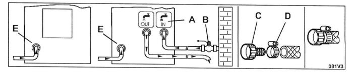
Use linen- rubber tubes for water connection, arranged for 15 Bar pressures, interposing a valve or a faucet [B] ABOVE the delivery pipe; use a 3/4" rubber holder [C], well fixed with a proper band [D] to connect the tubes at the device's union.
