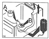
This safety device, composed of an approved magnet [1] and of a magnetic contact [2] is aimed at avoiding any accidents provoked by the stirrer starting accidentally. Consequently, this machine does not work without a magnet. In case the magnet [A] or the rotor lid [B] are removed, the stirrer stops working immediately.
