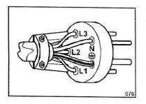
A 5 pole (400V- 415V-  $3\sim$ ), or 4 pole (200V- 220V-  $3\sim$ ), or 3 pole (230V-  $1\sim$ ) plug, suitable with the current socket, must be installed at the end of the device's power supply cable.
