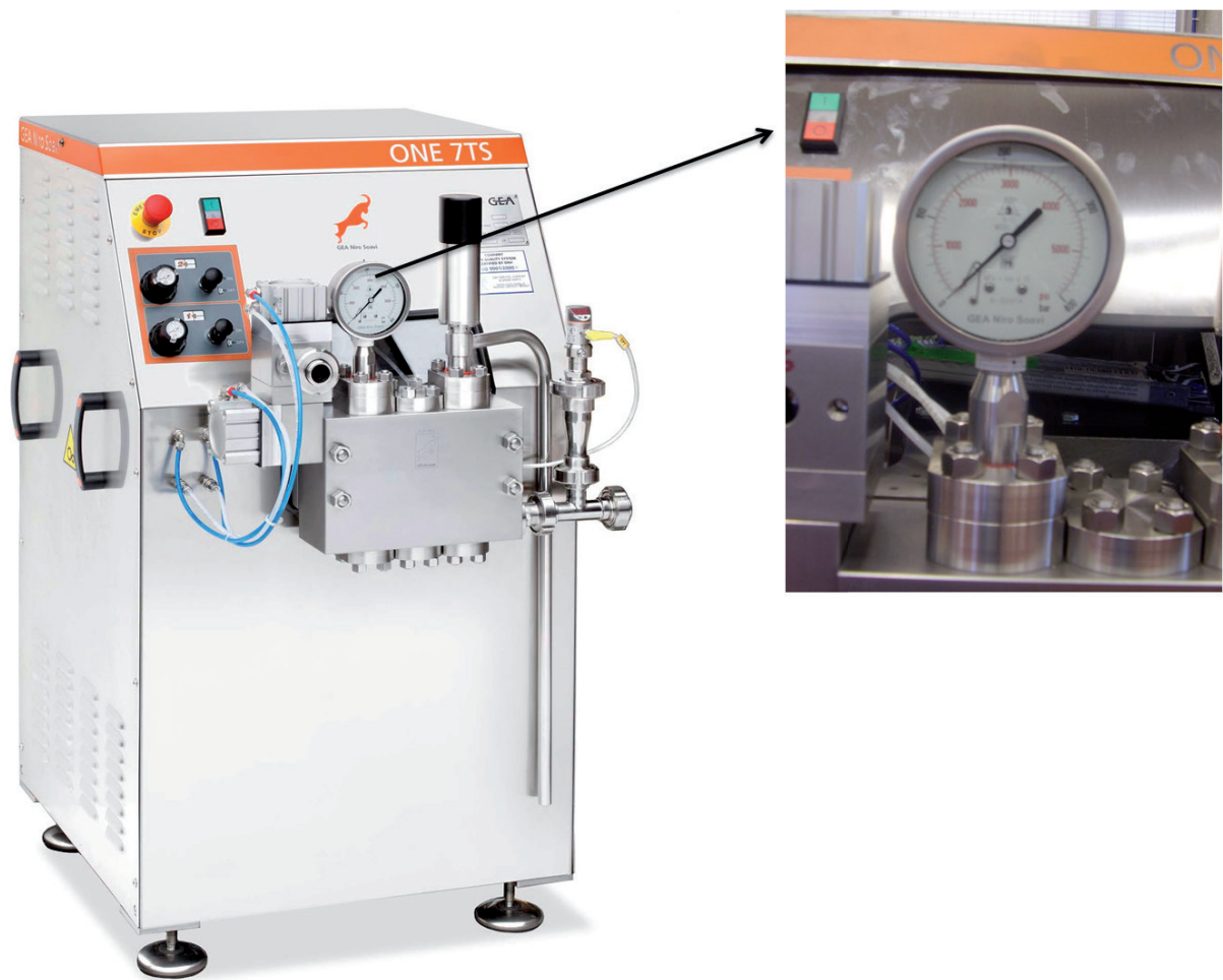
FIRST STAGE HEAD PRESSURE GAUGE FIG. 2.5
