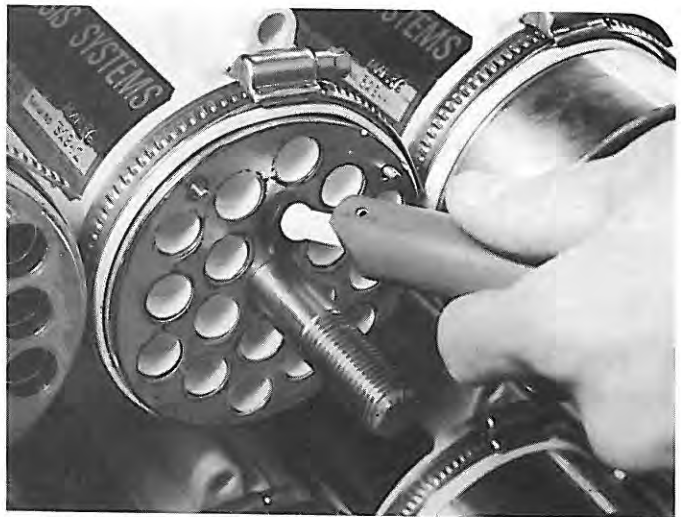
8. Straighten seal with tool provided. Chamfer on tool enables seal to be held in place as tool is withdrawn.
