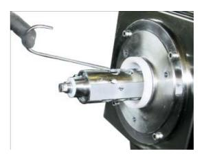
3 Remove the ice-cream pressure manometer and the mixture inlet line.
