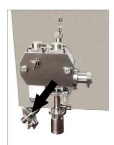
3 Connect the CIP system return line to the cylinder outlet;
