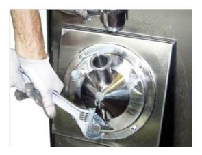
2 Remove the DASHER from the cylinder using the extractor tool supplied as standard, as shown in the following figure.
