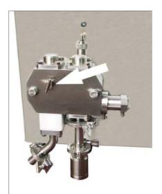
If a centrifugal pump is installed between the freezer pump and the vat, start the freezer pump only after bleeding the entire line (vat – centrifugal pump and centrifugal pump - freezer).
