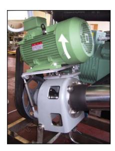
If the direction is incorrect, swap two of the phases in the power line.
