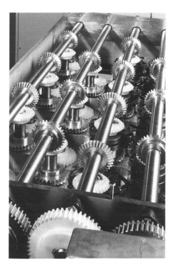
View of gearbox controlling the drive and sealing rollers for fin sealing.
