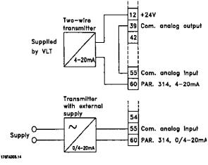
Parameter 314 = *Reference* [1], *Feedback* [2] Parameter 315 = *Terminal 60, min. scaling* Parameter 316 = *Terminal 60, max. scaling*
