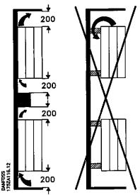
All Compact units in the above-mentioned series require a minimum space of 200 mm above and below the enclosure and must be installed on a plane, vertical surface (no spacers). This applies to both IP 20 and IP 54 units.
