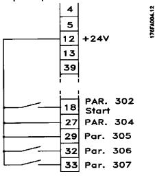
Speed up and down using terminals 32 and 33.
