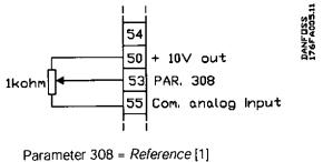
Parameter 309 = Terminal 53, min. scaling Parameter 310 = Terminal 53, max. scaling
