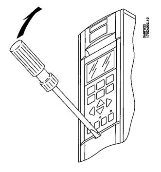
Once the protective cover has been removed, the actual EMC-correct installation can start. See drawings on pages 30-32.
