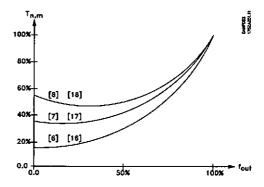
Choose the torque characteristics giving the most reliable operation, the lowest possible energy consumption and the lowest acoustic noise. Select Special motor characteristics if a special U/f setting is required to match the motor in question. Set the break points in parameters 422-432.
