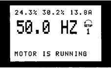
In this state, data values for four operating values are shown at the same time, giving the related unit, cf. table. In the example, Reference, Torque, Current and Frequency are selected as variables in the first and second line.
