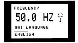
The 3rd line of the display shows the parameter number and name, while the status/value of the selected parameter are shown in line 4.
