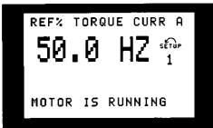
This is where parameter names and units for operating variables in the first and second line are given operating variable 2 remains unchanged.
