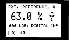
Free a data-log if there is a trip and release it when resetting the VLT frequency converter. Data-logging is active when the motor is running.
