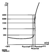
If a motor features a KLIXON thermal switch instead, this can also be connected to the input. If motors run in parallel, the thermistors/thermal switches can be connected in series (total resistance < 3 kohm).
