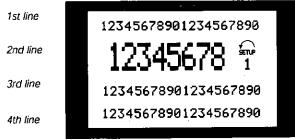
1st line shows up to 3 measurements continuously in normal operating status or a text which explains the 2 nd line.
