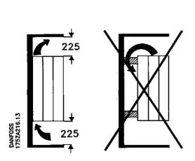
All Compact units in the above-mentioned series require a minimum space of 225 mm above and below the enclosure and must be installed on a plane, vertical surface (no spacers). This applies to both IP 00, IP 20 and IP 54 units.
