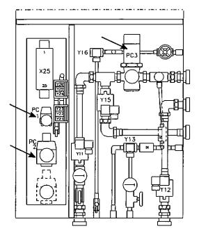
Air reducing valves PC1 and PC2 Water reducing valve PC3
