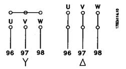
Normally, small motors are star-connected (200/400 V, Δ/Y).
