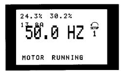
The selected programming setup number will flash to the right of the active setup.
