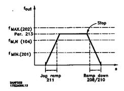
The jog ramp time starts if a jog signal is given via the control panel, the digital inputs or the serial communication port.
