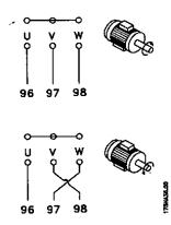
The factory setting is for clockwise rotation with the VLT frequency transformer output connected as follows.
