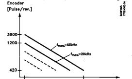
The encoder used is to be of the Open Collector PNP 0/24 V DC type (max. 20 kHz) or a Push-Pull circuit 0/24 V DC (max. 65 kHz).
