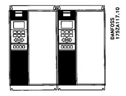
All Compact units can be installed side-by-side without any space between them, since the units do not require any cooling on the sides.
