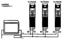
In order to avoid potential equalizing currents in the screen, the cable screen can be earthed via terminal 61, which is connected to the frame via an RC-link.
