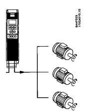
VLT 5000 Series is able to control several motors connected in parallel. If the motors are to have different rpm values, the motors must have different rated rpm values. Motor rpm is changed simultaneously, which means that the ratio between the rated rpm values is maintained across the range. The total current consumption of the motors is not to exceed the maximum rated output current  $I_{VLT,N}$  for the VLT frequency converter.
