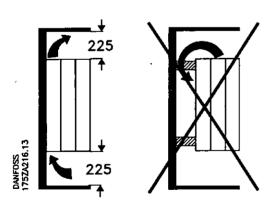
All Compact units in the above-mentioned series require a minimum space of 225 mm above and below the enclosure and must be installed on a plane, vertical surface (no spacers). This applies to both IP 00, IP 20 and IP 54 units.
