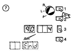
8) Set the mode selector switch in position L or R, whichever applicable, when the parameter value(s) is/are set.
