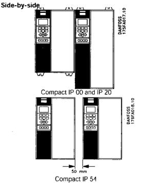
All IP 00 and IP 20 units in the above-mentioned series can be installed side by side without any space between them.
