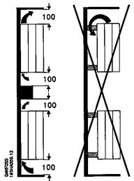
All Compact units require a minimum space of 100 mm above and below the enclosure and must be installed on a plane, vertical surface (no spacers). This applies to both IP 20 and IP 54 units.
