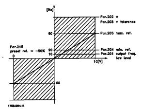
Parameter 200 Output frequency range/direction = both directions.
