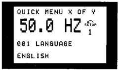
At the bottom of the display, the parameter number and name are given together with the status/value of the first parameter under Quick Setup. The first time the [Quick Menu] key is pressed after the unit has been switched on, the read-outs always start at pos. 1 - see table below.
