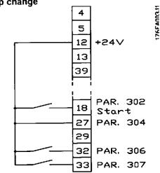
Selection of setup using terminals 32 and 33.
