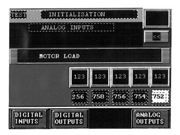
Note that is is only possible to monitor the status of the analog inputs. No forcing is possible. The value og the analog inputs are all scaled from 0-100 %.
