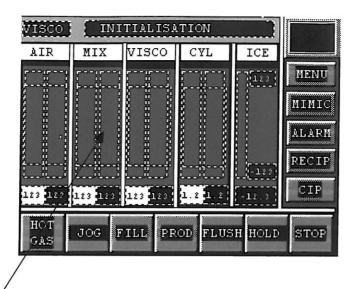
By pressing the middle of the bar graph area on the mix flow controller, indicated as a rectangle on the picture above, you will enter into the mix flow set-up screen where it is possible to adjust the various parameters related to the mix flow control loop.
