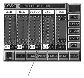
By pressing the middle of the bar graph area on the cylinder pressure controller, indicated as a rectangle on the picture above, you will enter into the Cylinder pressure set-up screen where it is possible to adjust the various parameters related to the Cylinder Pressure control loop.
