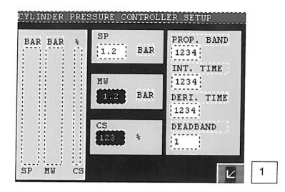
On the bar graph area on the left of the screen the set point, the current measured cylinder pressure and the control output to the product pump inverter is represented
