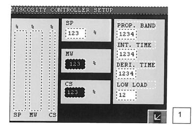
On the bar graph area on the left of the screen the set point, the current measured motor load value and the control output to the backpressure valve is represented. Please note that all bar graphs are shown as percent of full-scale range of the freezer.
