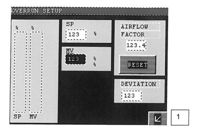
The bar graph area on the left of the screen shows the overrun set point (SP) and the current overrun measured Value (MV) in percent. Please note that even if the set point is white it is not possible to change it.
