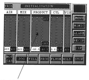
By pressing the middle of the bar graph area on the product temperature controller, indicated as a rectangle on the picture above, you will enter into the product temperature tuning screen where it is possible to adjust the various parameters related to the control loop.
