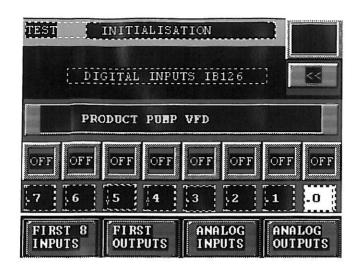
By pressing <first 8 inputs > the status screen for the first 8 inputs will be displayed. By pressing first outputs the first 8 outputs of the freezers PLC will be displayed:
