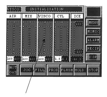
By pressing the middle of the bar graph area on the viscosity controller, indicated as a rectangle on the picture above, you will enter into the motor load set-up screen where it is possible to adjust the various parameters related to the mix flow control loop.
