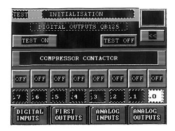
By pressing <first outputs> the first outputs of the freezers PLC will be displayed. By pressing <analog inputs> the analog inputs of the freezers PLC will be displayed:
