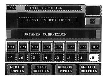
This is the first of the test screens. It is showing the status of the first 8 inputs of the freezers PLC. By pressing the numbers from 0 to 7 an explanation is clear text is displayed in the message field. It is not possible to force the status of an input.
