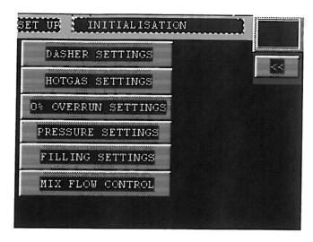
By pressing the various buttons on the general set up screen the adjustable parameters pops up on the screen.
