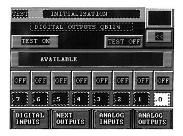
By pressing the <test on> button it is possible to force the status of the outputs. This is only possible when the freezer is in idle mode.
