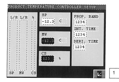
On the bar graph area on the left of the screen the set point, the current measured temperature and the control output to the backpressure control valve is represented. Please note that set point and measured value bar graphs are shown in engineering units while the control output bar graph is in percent of full scale.
