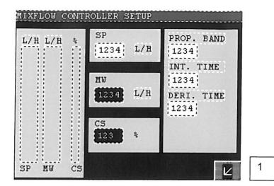
On the bar graph area on the left of the screen the set point, the current measured mix flow value and the control output to the mix pump inverter are represented.
