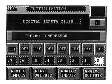
By pressing <next 8 inputs the status screen for the next 8 inputs will be displayed:
