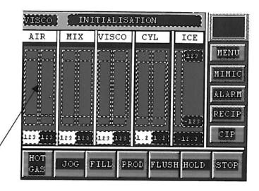
By pressing the middle of the bar graph area on the overrun controller on production screen, indicated as a rectangle on the picture above, you will enter into the overrun set-up screen where it is possible to adjust overrun parameters.
