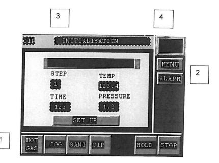
On the cleaning screen it is possible to start/stop and supervise the cleaning and sanitizing sequences.
