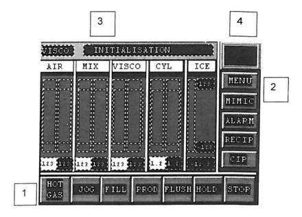
This screen is the normal production screen when the freezer is set-up for viscosity production. The screen is divided into the status indication part, the controller area, the main command panel and the operator navigation panel.
