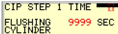
On this screen you set the step 1 time for the CIP sequencer. By pressing K7 (Arrow) up you increase the time and by pressing K8 (Arrow Down) you decrease the time. Keeping the keys pressed will make the adjustments go faster and faster. The setpoint adjustment is immediately being stored. There is no need for acknowledging the adjustment.
