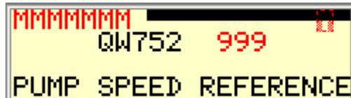
On this screen you can see the status of the first analog output in the PLC. The output range goes from 0 to 100 percent, which is converted in the PLC's analog output module to 4 to 20 mA. This analog output is controlling the speed of the pumps
