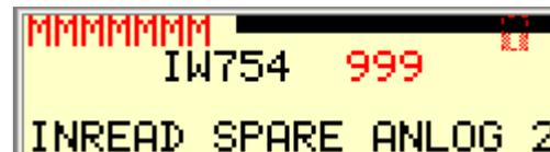
On this screen you can see that status of the second analog input in the PLC. The input range goes from 4 to 20 mA and this range is converted in the PLC from 0 to 100 Percent. This analog input is not used at present.
