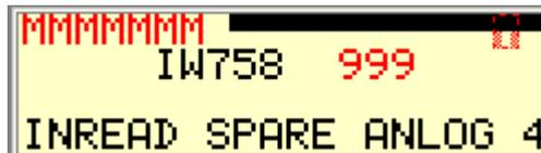
On this screen you can see that status of the third fourth input in the PLC. The input range goes from 4 to 20 mA and this range is converted in the PLC from 0 to 100 Percent. This analog input is not used at present.
