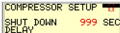
When the Compressor is stopped there should be a small delay in order to make sure that the evaporator is emptied for Halo Carbon. This parameter sets the stop delay.
