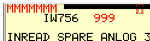
On this screen you can see that status of the third analog input in the PLC. The input range goes from 4 to 20 mA and this range is converted in the PLC from 0 to 100 Percent. This analog input is not used at present.
