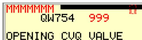
On this screen you can see the status of the second analog output in the PLC. The output range goes from 0 to 100 Percent which is converted in the PLC's analog output module to 4 to 20 mA. This analog output is controlling the opening of the freezers backpressure valve.
