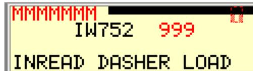
On this screen you can see that status of the first analog input in the PLC. The input range goes from 4 to 20 mA and this range is converted in the PLC from 0 to 100 Percent. The analog in-read value is from the dasher load current transducer.
