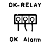
Fig. 26 : OK relay (always normally-energized)
