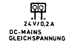
Fig. 20: Power supply + 24V DC
