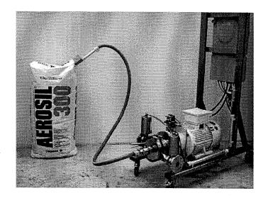
TDS-machines may be used for all processing steps, from the barrel emptying, powder transportation, wetting and dispersing up to a complete desagglomeration. This offers a very high potential in rationalisation
