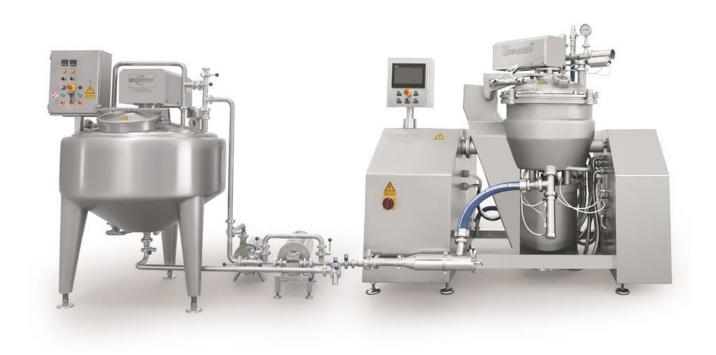
$\begin{array}{c} \textbf{MULTIFUNCTIONAL INDUSTRIAL MIXER CCM-200 WITH OPTIONAL AUXILIARY EQUIPMENT} \\ & (\texttt{LINE OPTION}) \end{array}$
