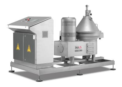
THE PRODUCT MAXCREAM 10T is a centrifugal separator configured as a concentrator for dairy application, with double paring discs, partial and total automatic discharge capabilities, and ready for Clean-In-Place (CIP).
