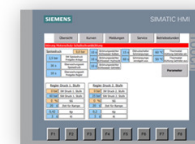
Touch panel for homogenizer control
