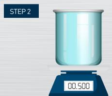
Fill the container with un-frozen liquid mix right to the brim and place on the scales.
