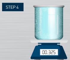
Place the container of frozen product on to the scales. Make a note of the weight of the frozen mixture.
