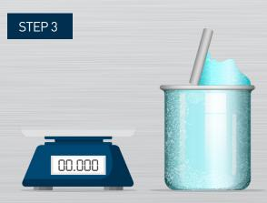
Clean and dry the container. Fill the container with frozen product directly from the machine; with a straight edge, level the top off.
