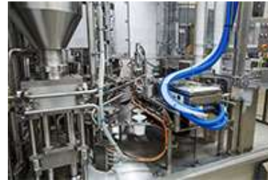
cup sterilization with piston dosing system 2-fold in servo execution
