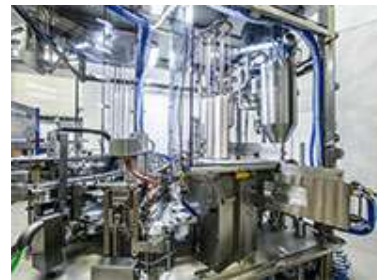
sealing lid sterilization station with laminar flow air hood with sealing station
