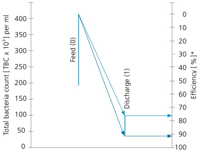
Fig. 7 Separation based on total bacterial count in modern bacteria-removing clarifiers (Here the efficiency is shown for the specific total bacterial count of 400,000 cells/ml)
