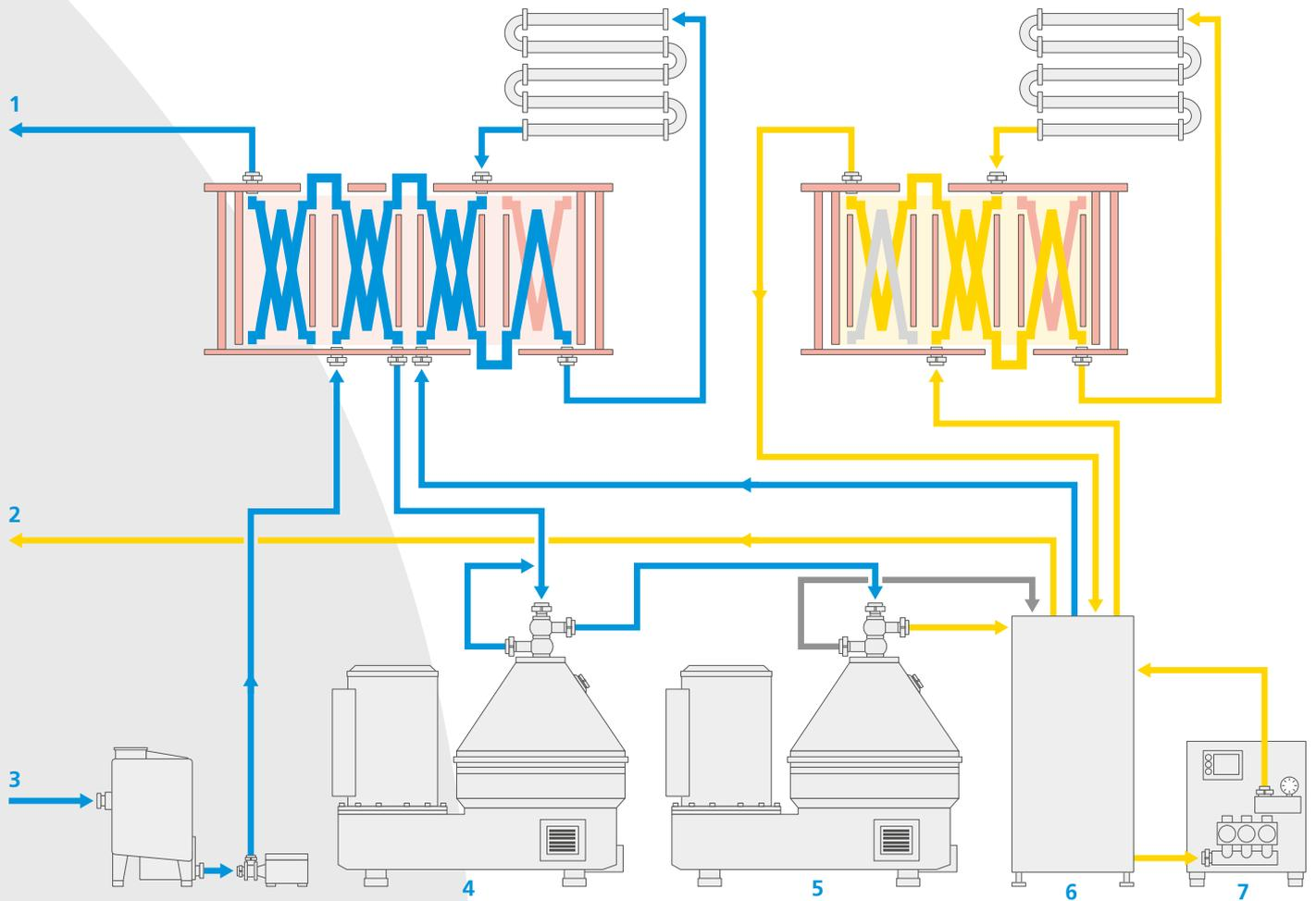
Fig. 8 Bacteria removal from fresh milk – Stage 1
