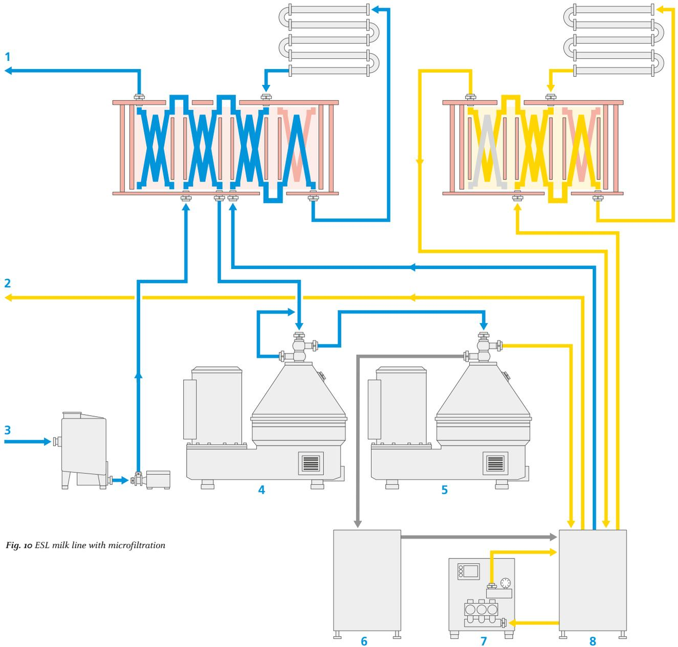
Fig. 10 ESL milk line with microfiltration
