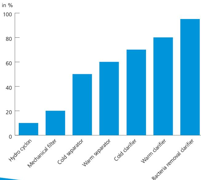
Fig. 1 Degrees of clarification in comparison
