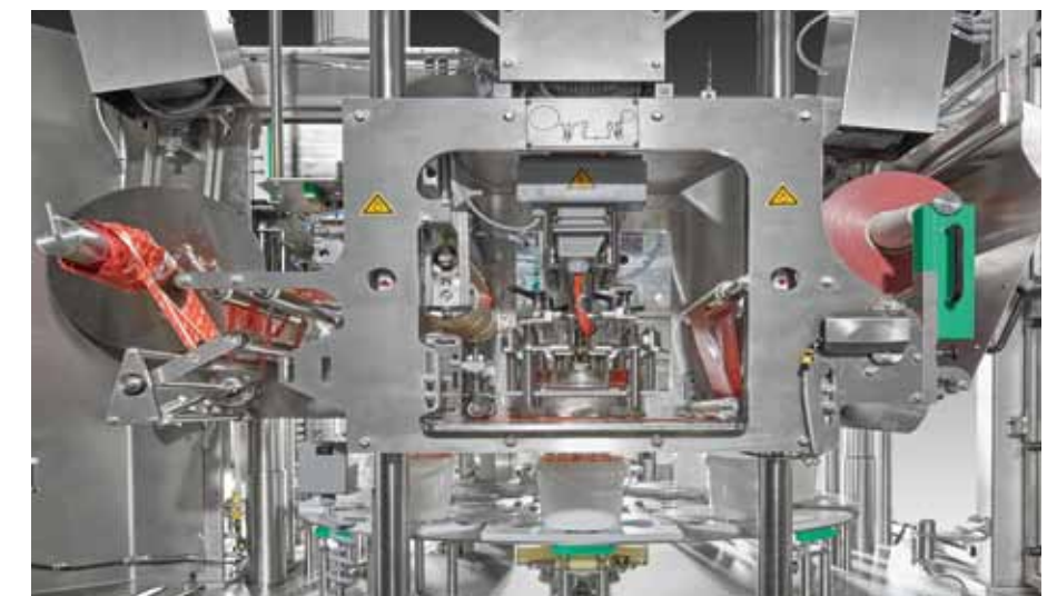
Cutting/sealing station for film from the reel
