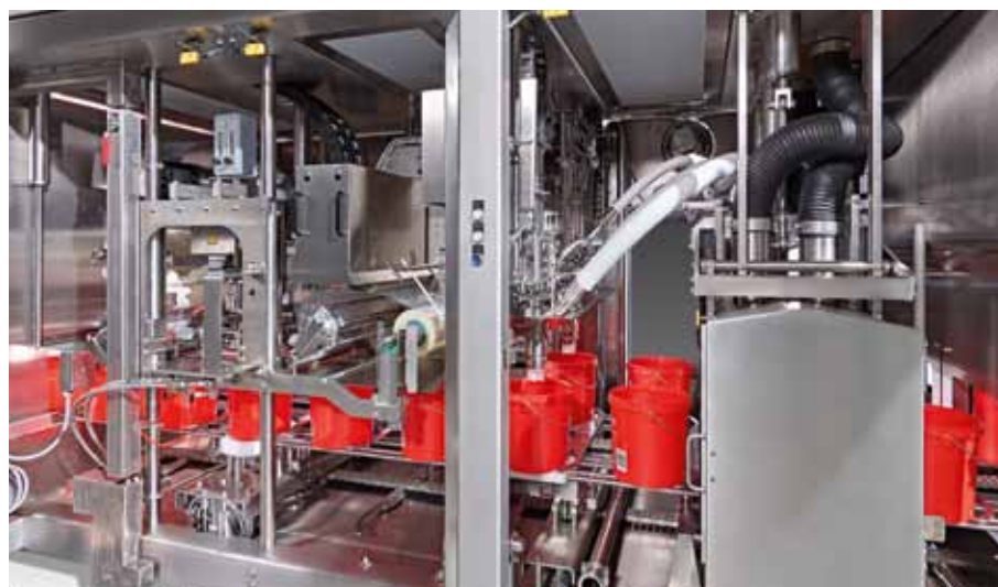
View into the inside of the linear bucket filler ERGOLINER XL
